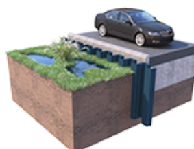
Cut-off walls used to protect places with variable or raised groundwater level
